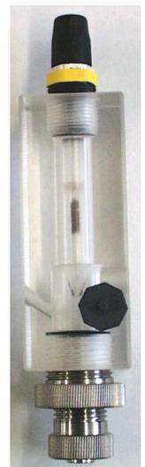
The active gold electrode consists of a gold round piece and is fitted within a stainless steel body which is working as the counter electrode, the measuring current flows between these two electrodes. This assembly is screwed from the bottom into the measuring cell. Blue glass beads moved by the measuring water are cleaning the surface of the gold electrode. The Ag/AgCl reference electrode is screwed from top.
